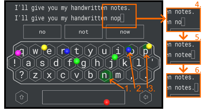
(b) Illustrated operation of the decoder’s coactivation detection and auto-correction components. 1: Intended ‘n’. 2: Intended ‘o’. 3: Coactivated ‘p’. 4: ‘p’ removed by coactivation module. 5: ‘tee’ entered by user. 6: Auto-correction of ‘notee’ to desired ‘notes’.
